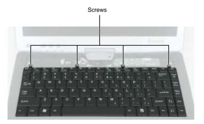
11 Lift the back edge of the keyboard, then slowly rotate it toward you so it lies **keys-down** on top of your convertible tablet PC. Be careful not to damage the LCD panel, or unplug the keyboard ribbon cable.
