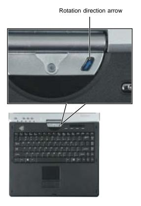
**3** Rotate the LCD panel in the direction of the rotation direction arrow until the panel is backwards. The panel *soft-locks* into the final position.
