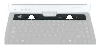
**10** With a small Phillips screwdriver, remove the four keyboard screws and put them in a safe place.
